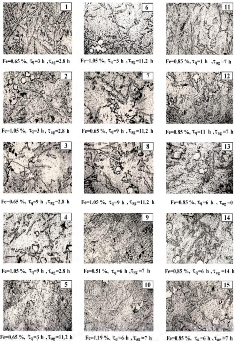
**Fig. 1.** The microstructure of the alloy AK8M3 according to the matrix design of experiments ( $\times 200$ ): 1...8 – plan of the matrix  $2^3$ ; 9, 10 – star points, 11...15 – points of the center of the plan (zero level of varying)
