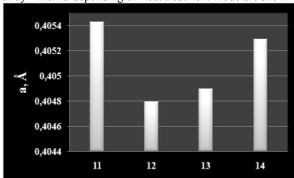
**Fig. 2.** The lattice parameter of a solid solution of aluminum in the alloy AK8M3.
