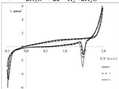
a) Cycle potentiodynamic curves (three cycles) obtained on the electrode with tape PbCa0.05Sn1.1.
