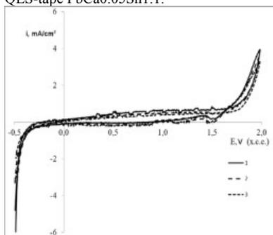
d) Cycle potentiodynamic curves (three cycles) obtained on the electrode with QLS-tape PbCa0.05Sn1.1 ,0.03 % Ba.
