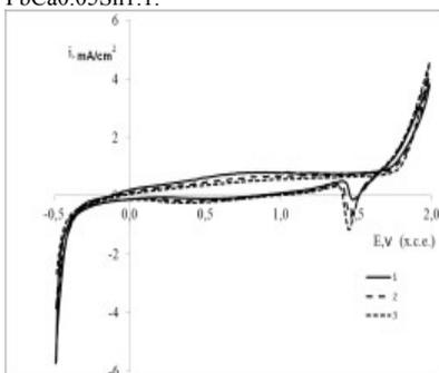
c) Cycle potentiodynamic curves (three cycles) obtained on the electrode with QLS-tape PbCa0.05Sn1.1 ,0.015 % Ba.
