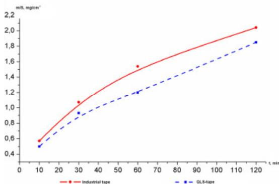
**Fig. 2** The dependence of a weight reduction of alloy electrodes from corrosion time
