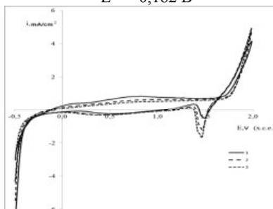
b) Cycle potentiodynamic curves (three cycles) obtained on the electrode m with QLS-tape PbCa0.05Sn1.1.
