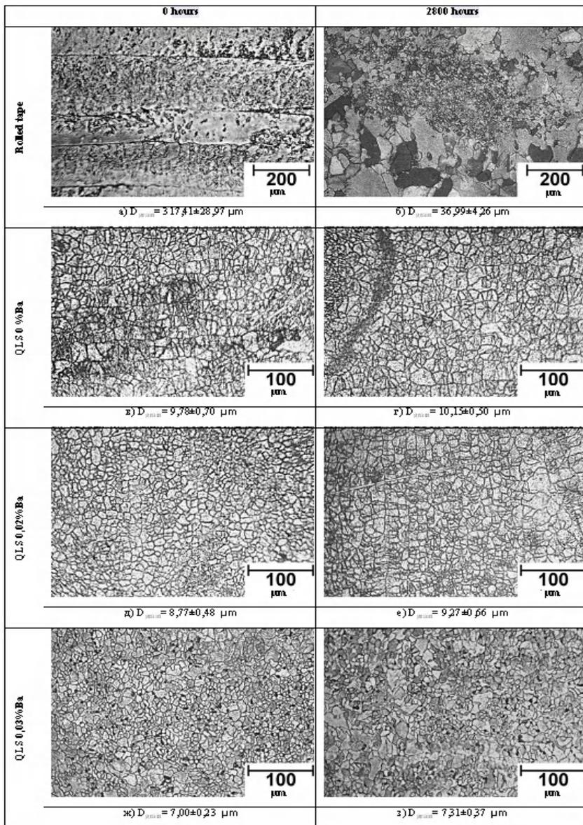
Fig. 1. The structures of the samples D – an average size of the grain
