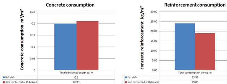
Fig. 10. Consumption of concrete  $m^3/m^2$  and reinforcement  $kg/m^2$  compressed zone.
