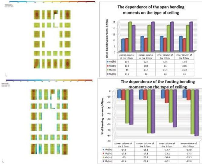
Fig. 7. Dependency of bending moments on the construction of the slab
