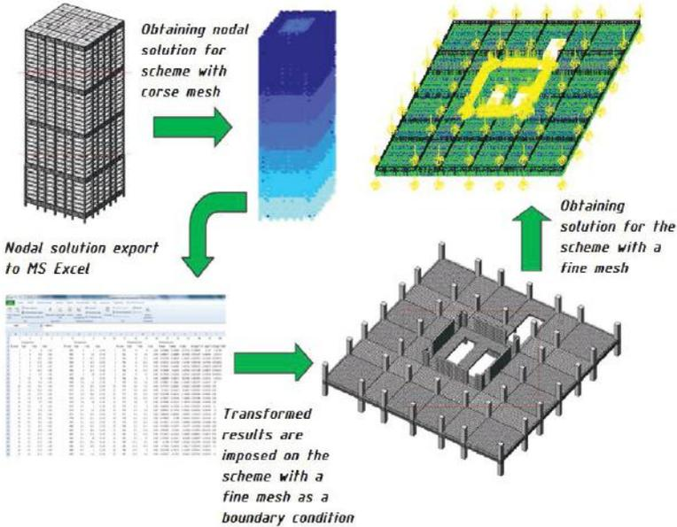
Fig 4. Fragmentation method implementation for «LIRA» software
