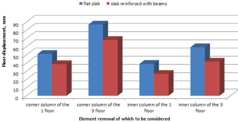
Fig.5. Dependency of construction displacement to the type of floor in case of progressive collapse
