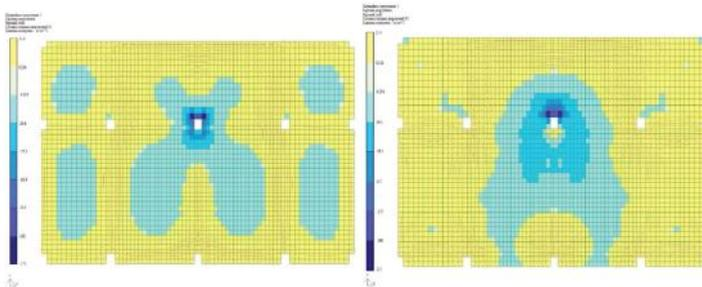
Fig. 8. Crack distribution in slabs adjacent to the damaged cells
