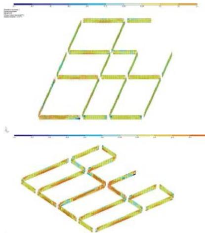
Fig. 9. Crack distribution in beams adjacent to the damaged cells
