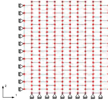
Fig. 1. 11 by 11 cell representing a symmetric quarter of the initial structure
