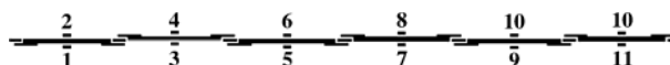
Fig. 3 – The placement of strain gauges on surface of flexible bottom chord of the steel and concrete composite cable space frame
