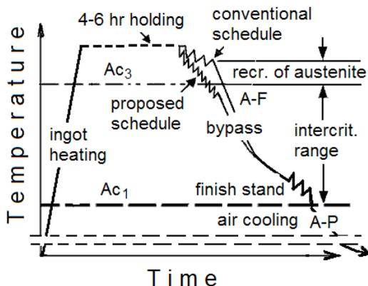
**Figure 1.** Conventional and proposed controlled rolling schedules.
