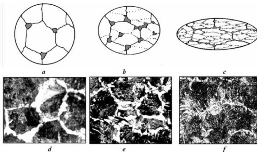
**Figure 2.** Sequential stages of  $\alpha$ -crystal nucleation at polygon boundaries at temperatures reduced down to the values below point  $A_{c3}$ ; *d – f*: precipitation of hypoeutectoid ferrite in steels which underwent austenite decomposition after cooling in air,  $\times 800$ : *d*: from a single heating by 1050  $^{\circ}\text{C}$ , *e*: after 16% hot reduction at 1000  $^{\circ}\text{C}$ ; *f*: after 36% hot reduction at 1000  $^{\circ}\text{C}$ .
