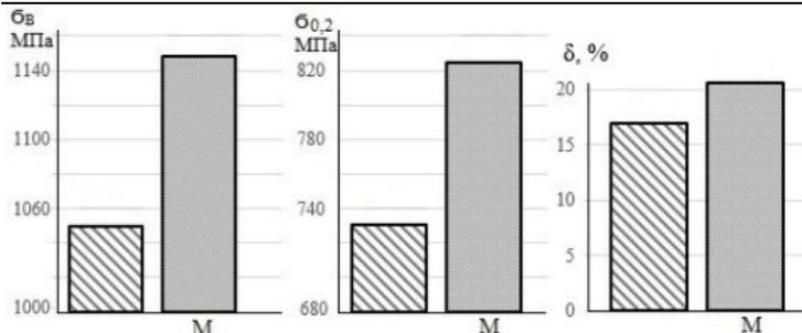
**Fig. 1.** The mechanical properties of heat-resistant nickel alloy XH59MBTKIOJ before and after modifying (M - modified alloy).
