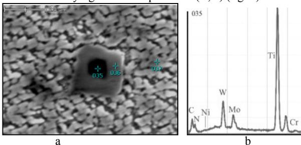
**Fig. 3.** The microstructure of the modified nickel alloy XH59MBTKIOJ, x 15000 (a), and the schedule of the intensity distribution of the characteristic radiation of elements (b).
