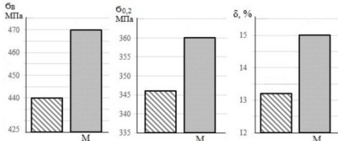
**Fig. 2.** Mechanical properties of 1570 aluminum alloy before and after modification (M - modified alloy).
