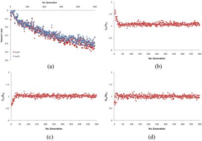
Fig. 5. Variations of Poisson's ratio, elastic modulus and shear modulus against number of generations
