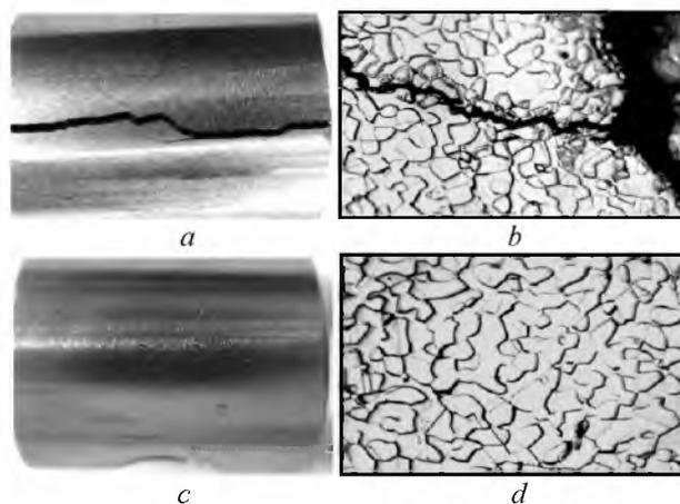
Рис. 9. Вид С-образных образцов холоднокатаной трубы (а,с) и их структуры (b, d,  $\times 500$ ) после закалок от ( $^{\circ}$ C): 1050 (а, b) и (1150+1050) (с, d) и испытаний на стойкость против КР / Appearance of C-shaped specimens taken from a cold-rolled tube (a, c) and their structure (b, d,  $\times 500$ ) after quenching from ( $^{\circ}$ C): 1050 (a, b) and (1150+1050) (c, d) and corrosion cracking resistance tests
